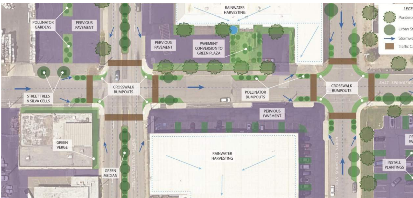
Figure 18. Concept for East Springfield living street elements including tree plantings, pollinator bumpouts, pervious pavement and rainwater harvesting features.
